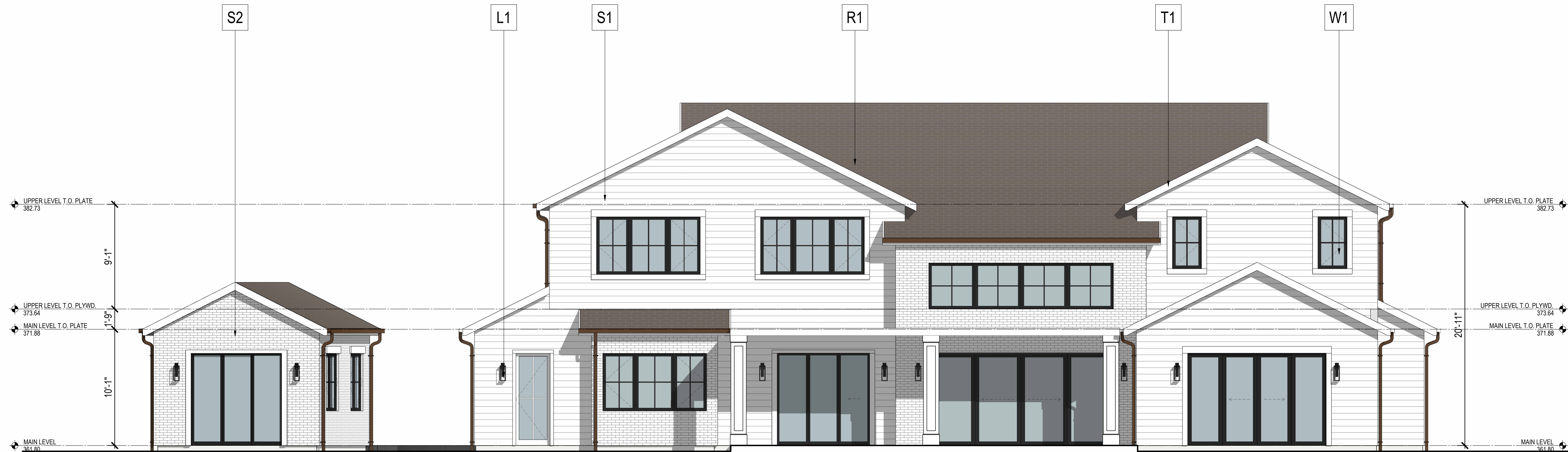
1 WEST ELEVATION 00 02 04 08 FEET 1/4" = 1'-0"
